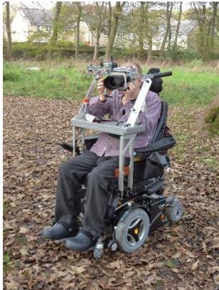
Austin Hughes, a volunteer with Remap Leeds set about finding a solution. He identified the key was to support the camera from above rather than below, making it inherently more stable. He built a camera mount which includes a base table, where Richard additionally keeps his mobile phone, and a cradle constructed from aluminium to support the camera itself. Steel counterweights ensure the camera is well balanced and camera positions can be fine-tuned through slotted or screw adjustment.
