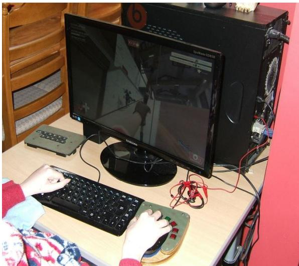
Martin, a volunteer with Remap Southampton realised that any solution would need to incorporate special switches that needed only the minimum of force to operate them. A suitable variety were sourced on the internet – ones that switch on and off very fast, making them ideal for this application. Martin developed a type of mouse mat that included the existing wireless mouse and the new switches buttons mounted in a way to suit the fingers on Brendon's right hand.
